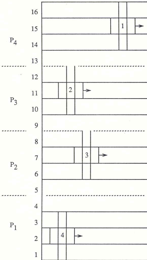
Fig. 2. Pipeline Model Using Four Processors each at a Different Iteration over the x-y Grid Space of a Reservoir
